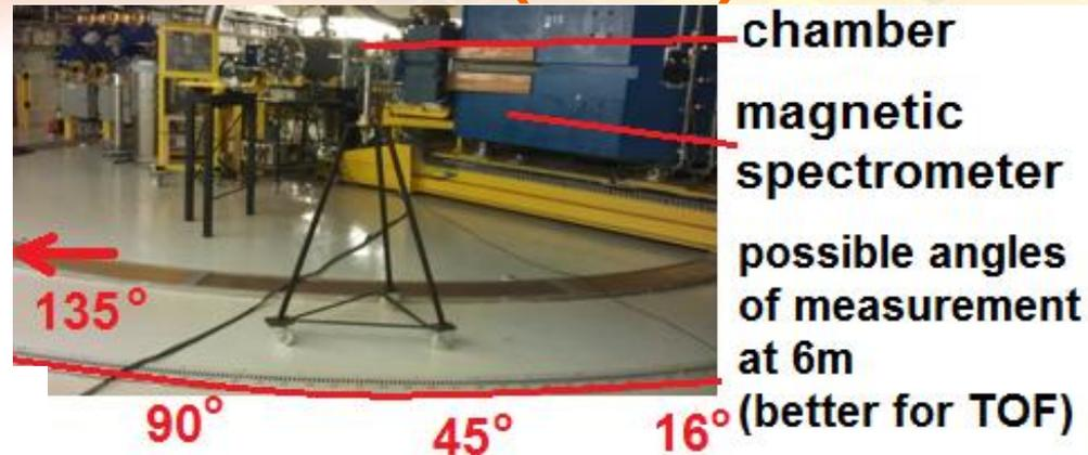
Figure 6: This is the iThemba LABS spectrometer vault showing collimated neutron beam holes at  $0^\circ$  and  $16^\circ$ . It shows the shielding which makes this facility the best for neutron measurements.
