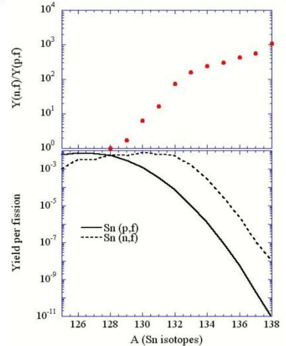
Figure 1: comparison of yields of proton induced fission for 70MeV protons (solid), and neutron induced fission for neutrons (dashed) for Sn isotopes. The upper plots give the yield ratios. Measurements done in the Holifield RIB Facility at Oak Ridge National Laboratory.
