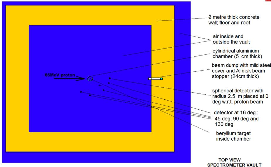
Figure 7: MCNPX geometry of the spectrometer vault with the chamber and beam dump
