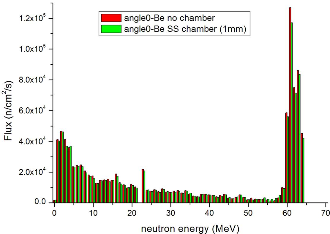
On the left are the results of the proposed chamber made of stainless steel (1mm thick) compared to the spectrum with no chamber. Results show that scattered neutrons from this chamber are negligible.
