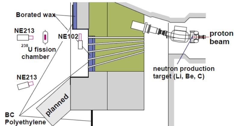
Figure 4: The sketch of the iTL neutron beam facility [4]
