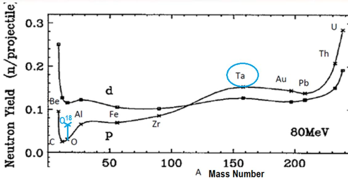
Figure 3: comparison of neutron yields induced 80MeV protons (p) and deuterons (d). Measurements done by Ridikas & Mittig at GANIL - France
