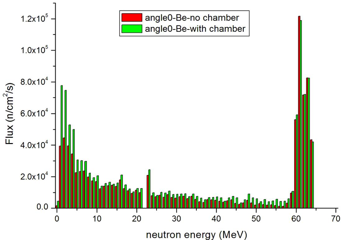
The effect of the spectrometer chamber simulation is shown on the left. The flux-energy distribution of neutrons produced by protons on Be with no chamber are calculated then compared to the Be inside the spectrometer chamber. The presence of the chamber considerably increase the neutron flux at low energies.
